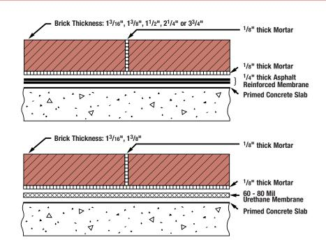
**Heavy Duty** — 2<sup>1</sup>/4-inch thick single brick for heavy trucking and extremely wet operations.
